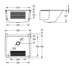
General purpose utility sink for wall mounting, stainless steel, surface satin finished, material thickness 0.9 mm, front panel with riffle, 1 1/2" flat perforated waste, prewelded mounting brackets.
