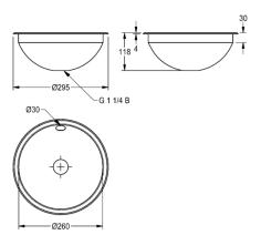
Round inset vanity basin, can be mounted from top or underneath, stainless steel, material thickness 1 mm, bowl diameter 260 mm, with overflow, inclusive 5/4" overflow kit without waste, stainless steel lugs for underneath mounting are included.
