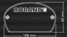
Dimensions for fabricator quartz heating and infra-red heating assemblies (HUQ & HUE)
