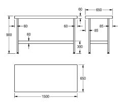
Centre tables at 900 mm height to complement the Mini, Midi and Magnum wall tables. The tables are manufactured from 1.2 mm thick, grade 1.4301 (304) stainless steel with a satin polish finish. The stainless steel underframe and shelf is supplied flat pack with easy to read assembly instructions. Each leg is fitted with an adjustable foot (-20, +10 mm) with a working height of 900 mm.
