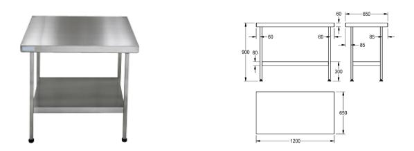
Centre tables at 900 mm height to complement the Mini, Midi and Magnum wall tables. The tables are manufactured from 1.2 mm thick, grade 1.4301 (304) stainless steel with a satin polish finish. The stainless steel underframe and shelf is supplied flat pack with easy to read assembly instructions. Each leg is fitted with an adjustable foot (-20, +10 mm) with a working height of 900 mm.
