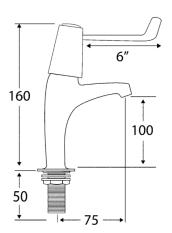
Lever operated pillar taps for connecting to hot and cold water. Supplied with 6" long levers which can be operated with a closed fist or wrists using a quarter turn action. Manufactured from chromium plated brass. A wall mounted elbow is available (sold separately).
