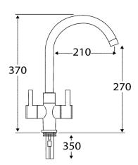
Monobloc mixer tap for connecting to hot and cold water. The 13 mm is ideal for those locations where there is only a single tap hole available. The operation of the F1059 monobloc mixer tap is carried out by a quarter turn ceramic disc which ensures a longer working life. Manufactured from chromium plated brass.
