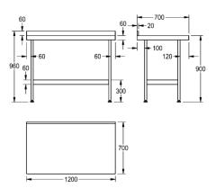
Magnum wall tables ideal to sit alongside the Magnum range of catering sinks. The mini wall tables are manufactured from 1.2 mm thick, grade 1.4301 (304) stainless steel with a satin polish finish. The stainless steel underframe and shelf is supplied flat pack with easy to read assembly instructions. Each leg is fitted with an adjustable foot (-20, +10 mm) with a working height of 900 mm.
