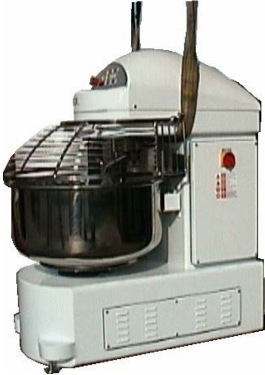
Fig. 4.1: Lifting with ropes
