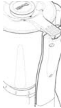
Fig. 2 Safety Interlock System
